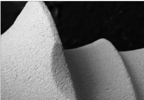
Fig.3 - Superficial topography by SEM that highlight the clean surface without residues.
