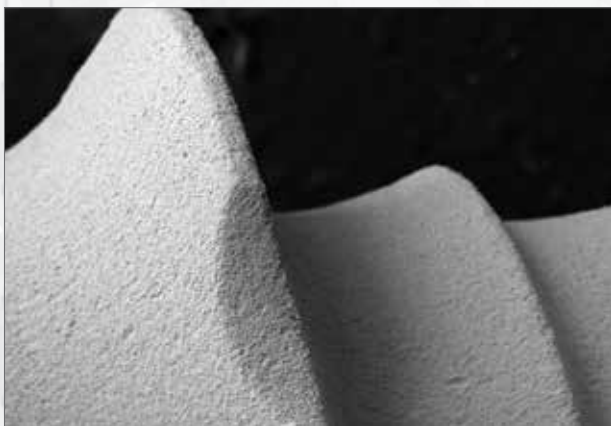
Fig.3 - Surface topography by SEM which highlight the clean surface without residues.
